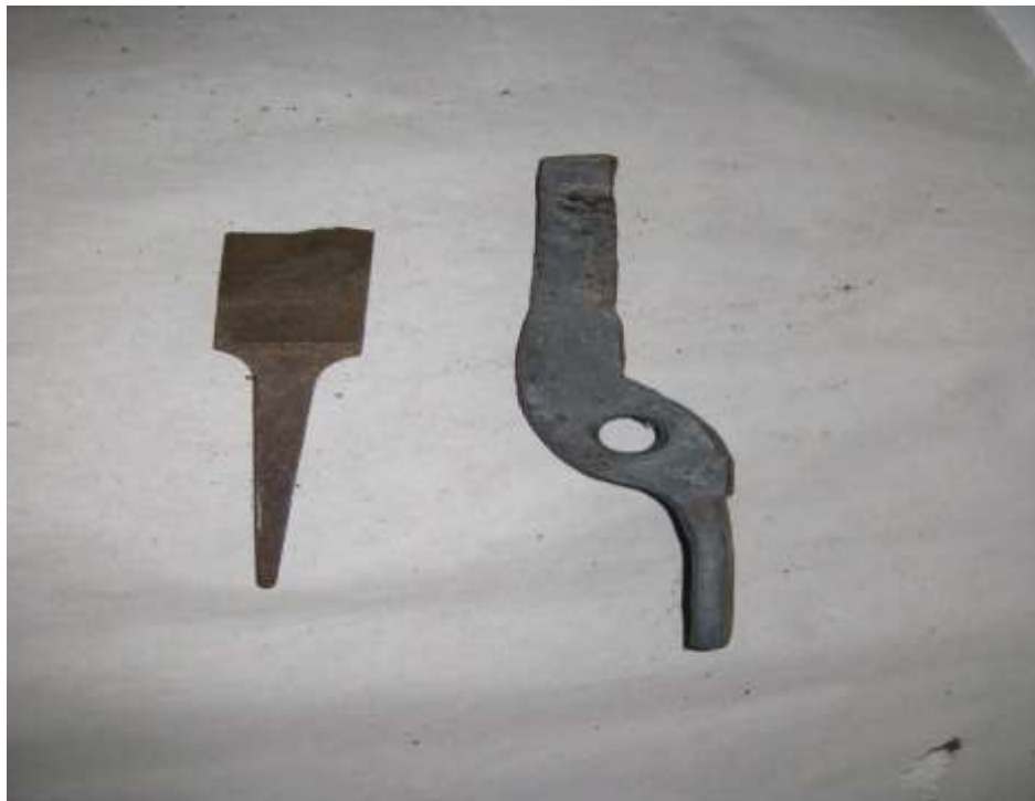
Figure 10: Discarded tool scraps. A broken file tang and a tong jaw. Since file was higher carbon tool steel, the remainder of the tool may have been the retained in the shop to be repurposed into another tool.
