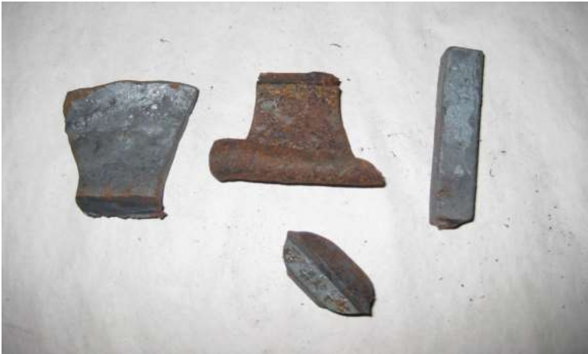
Figure 9: Scrap cut offs. Top row: two Scroll finials and square stock scrap. Bottom row: oval stock scrap. All were cut at forging heat using a Hardy.
