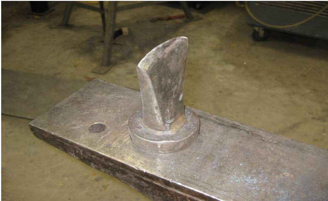
Figures 4 (above) and 5 (below): The Hardy is used to cut hot metal. The Hardy hole is used to hold numerous tools, e.g. the bending fork in Figure 3 but the cut off Hardy is the only one that is commonly referred to as “the Hardy”. Note the fish-tail end being cut off that will be discussed in Figure 6.
