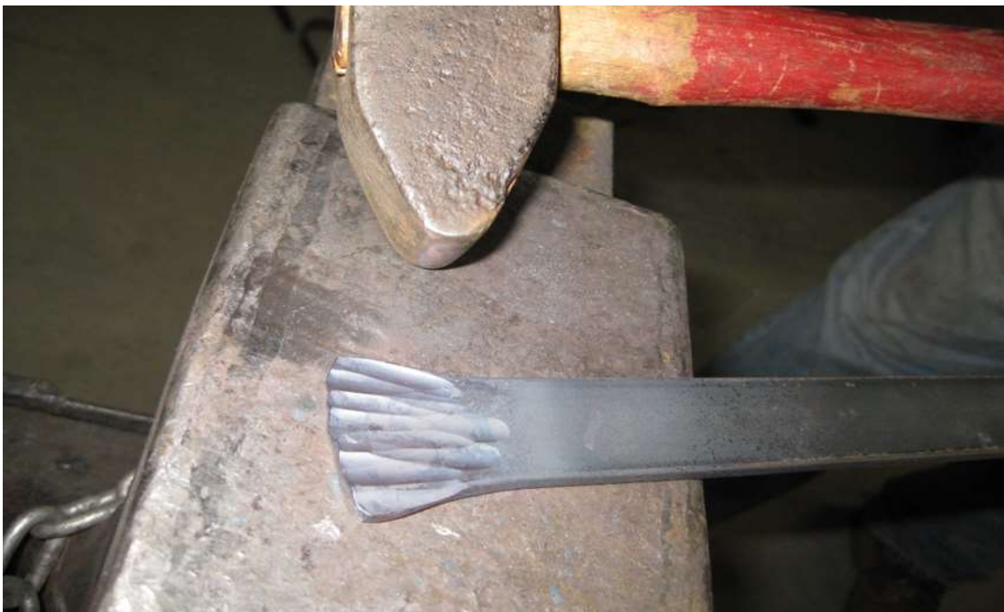
Figure 6: The fish-tail finial is a common decoration on hinges, scrolls, etc. It is made using the peen of a cross-peen hammer. Finials such as this are commonly found in scrap piles due to trimming of re-used stock.
