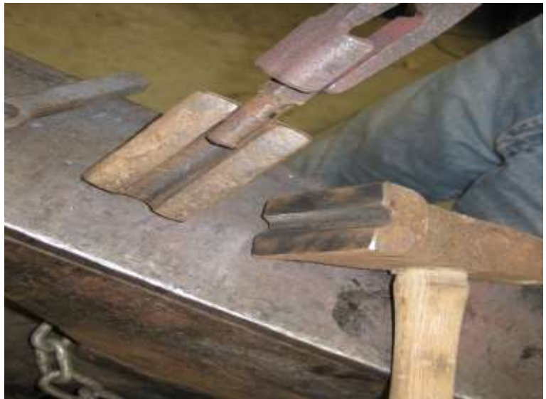
Figure 8: Top and bottom swages are used to neck down round or square hot stock to a smaller cross section. Note again that the top tool has a wooden handle and the bottom tool has a hardy shank.
