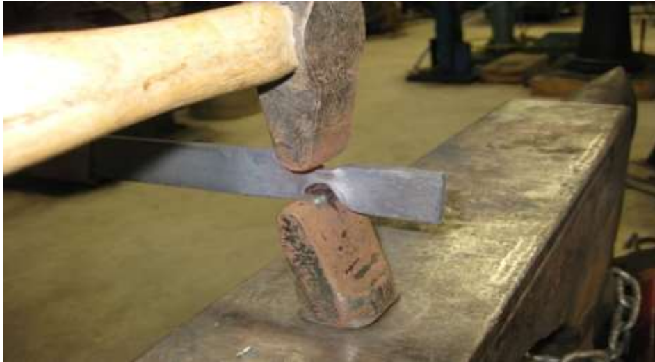
Figure 7: Top and bottom fullers being used to neck down hot stock. Top tools were often hafted with wooden handles which may rot before they are excavated. The bottom tools will have a square shank to fit the Hardy hole.
