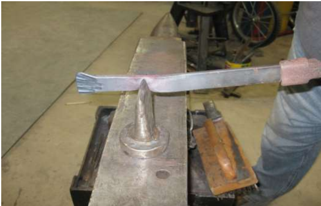
Figures 4 (above) and 5 (below): The Hardy is used to cut hot metal. The Hardy hole is used to hold numerous tools, e.g. the bending fork in Figure 3 but the cut off Hardy is the only one that is commonly referred to as “the Hardy”. Note the fish-tail end being cut off that will be discussed in Figure 6.
