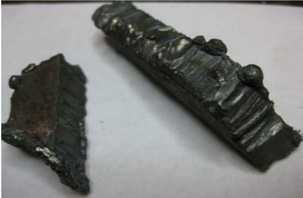
Figure 11: Scraps that were cut with a modern Oxyacetylene cutting torch. This technology came into common use in the early 20 th Century. Note the kerf marks burned into the steel by the hot gasses.
