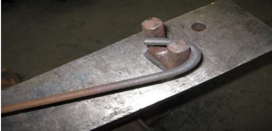
Figure 3: The bending fork is used in the Hardy hole to make controlled bends in hot stock.
